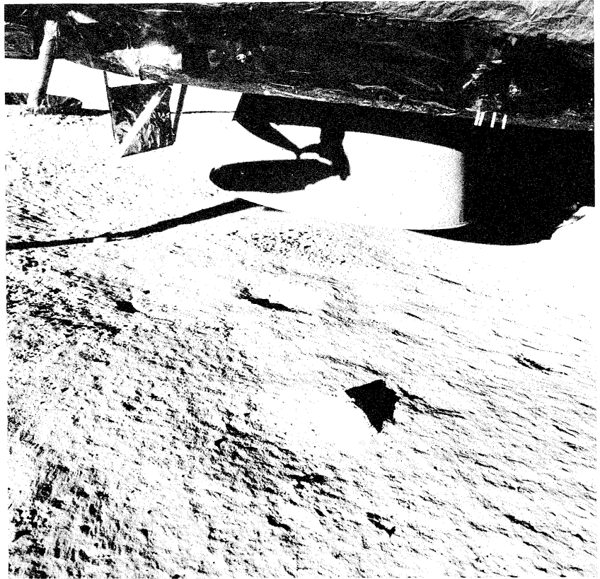
FIGURE 1-10.—The LM-inspection procedure included detailed examination and documentation of the surface materials eroded by the plume of the descent engine. The grooving that indicates radial transport of material from the point below the engine is evident. The erosion did not destroy small craters under the engine bell. The prominent rock in the foreground was later collected as a sample (AS14-66-9261).
