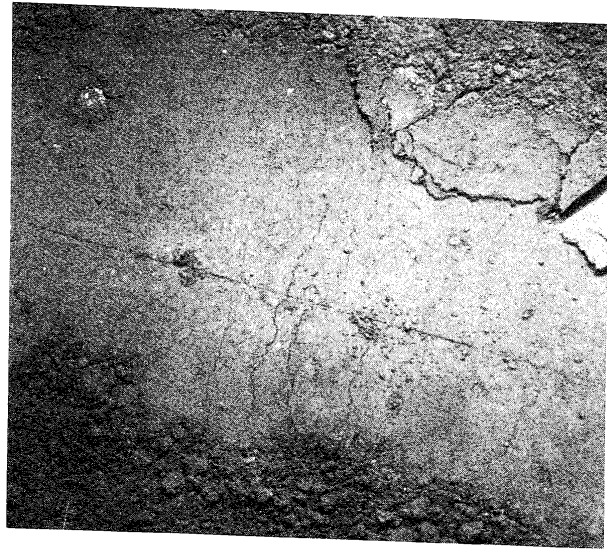
FIGURE 4-10.—The MET has evidently rolled across slightly firmer soil, because the track is narrower than before, which indicates less sinkage. In addition, there has been considerably less tendency for the soil to adhere to the tire, although fine cracks cross the track transverse to the direction of motion. A small white rock has been pushed into the soil by the MET tire in the upper left-hand corner of the photograph. The indentation at the upper right-hand corner of the photograph was probably produced by the edge of the camera while it was being positioned (AS14-77-10358).
