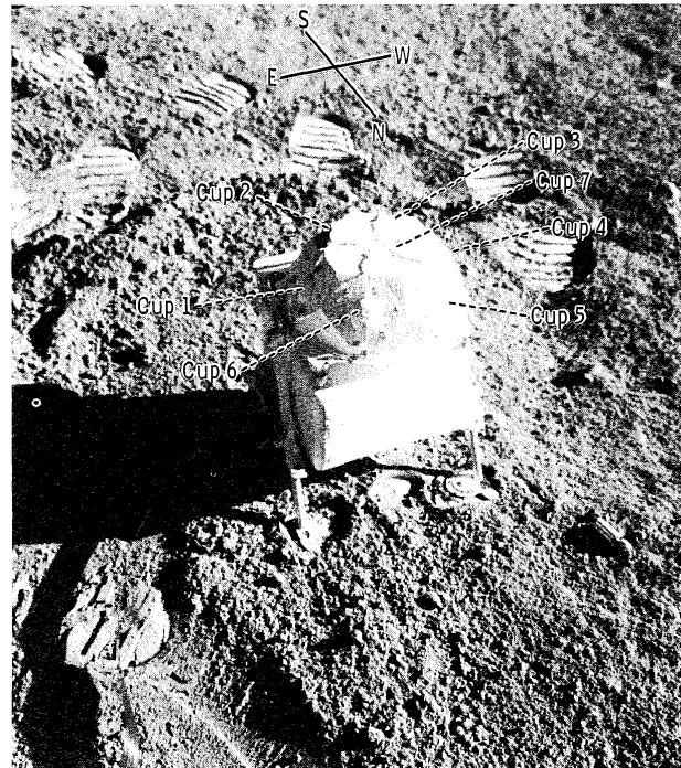
FIGURE 10-4.—Solar-wind spectrometer experiment as viewed from the south prior to dust-cover removal. Shadowing patterns, especially on the surface of cup 3, give information about orientation of the deployed instrument (AS15-86-11593).
