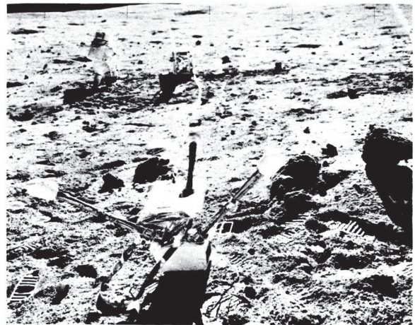
FIGURE 11-6.—The Apollo 16 LSM deployed on the Moon in the lunar highlands. Sensors are at the top ends of the booms and approximately 75 cm above the lunar surface.
