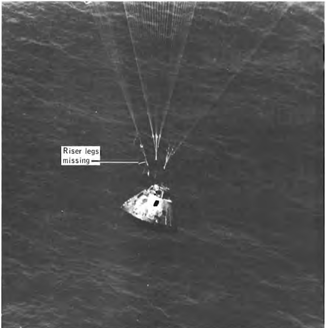
Figure 14-11.- Parachute riser damage noted during final descent.
