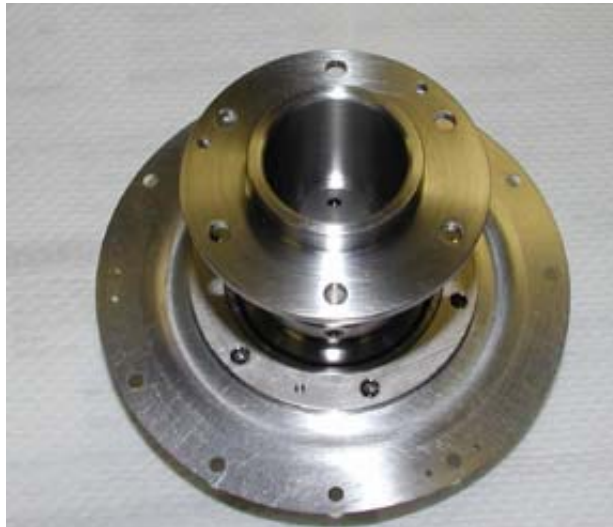
Figure 12. Hollow shaft after assembly.
