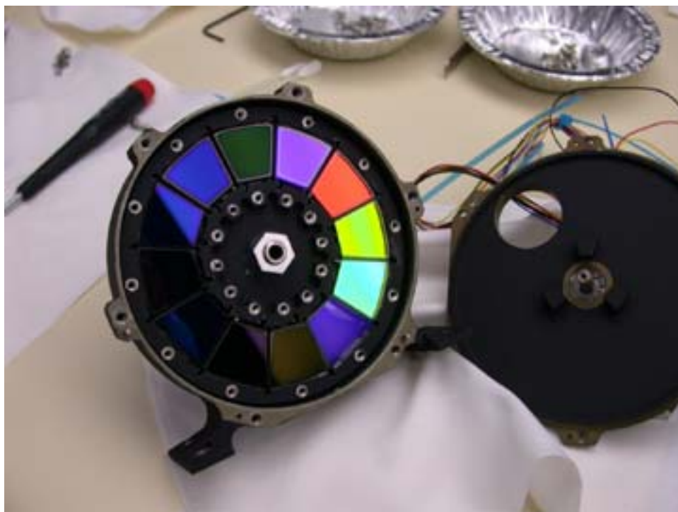
Figure 16. Filter wheel assembly
