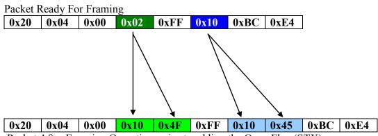
Packet After Escaping Operation, prior to adding the Open Flag (STX).
