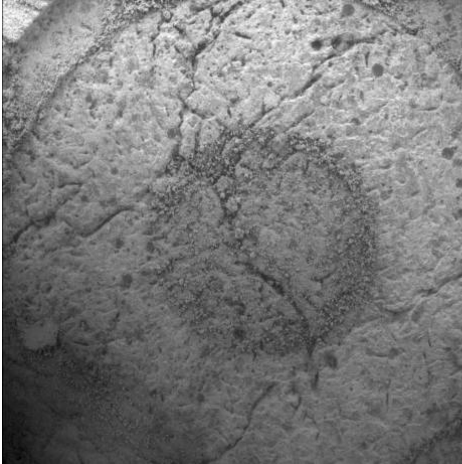
Figure 5. Opportunity MI image 1M245369672 of Rock Abrasion Tool target “Steno” acquired on Sol 1320 when target was fully shadowed. Lower response in lower left corner was not observed before the 2007 dust storm and was likely caused by dust contamination of the MI optics.
