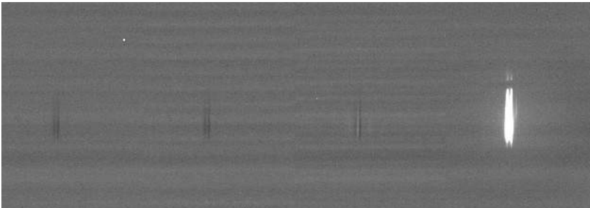
Weak electronics ghost negative images of the quadrant 4 signal in each other quadrant.
