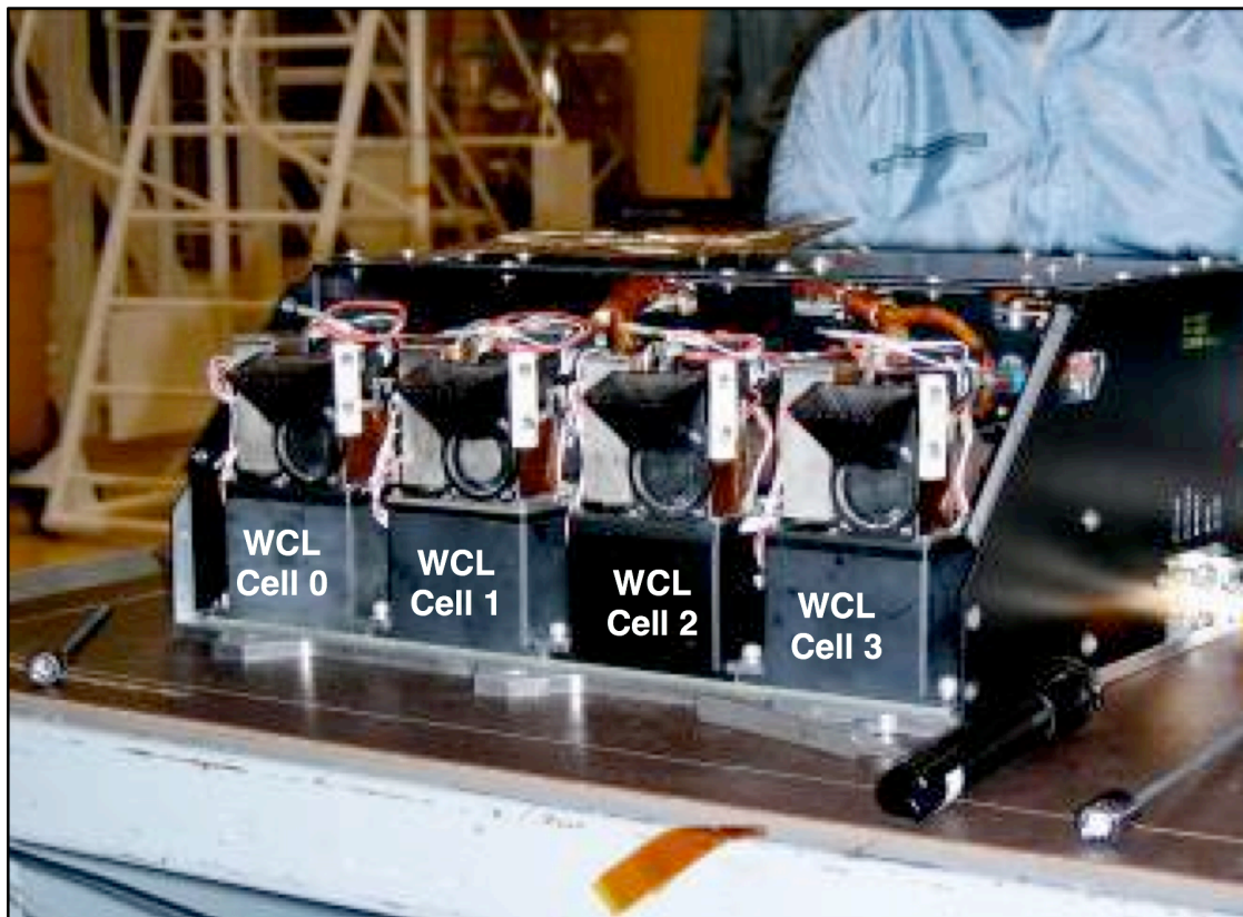
Figure 1. Photograph of MECA during ATLO at Lockheed-Martin just prior to integration onto the spacecraft. WCL Cell 0 is leftmost, near the OM sample entry. WCL cell 3 is right most, near the MECA external connectors.
