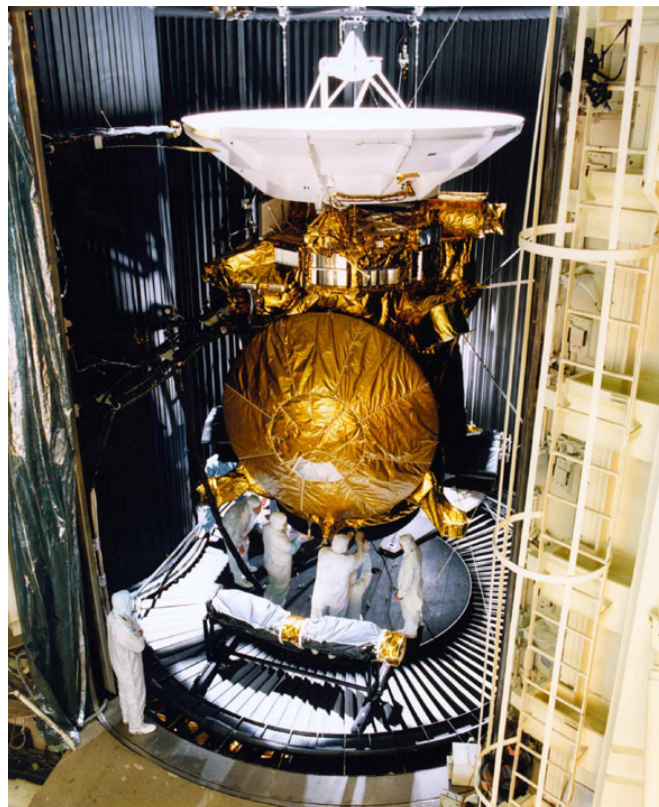
Figure 4: The Cassini spacecraft during pre-launch testing. Reference [37] gives a popular discussion of the Cassini mission, the spacecraft, and its instrumentation (photograph courtesy NASA/JPL-Caltech).
