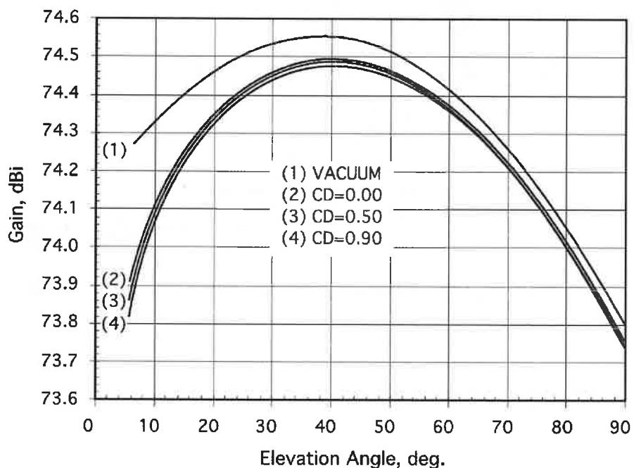
Figure 4. X-Band Receive Gain, DSS 14 Antenna, X-Only Configuration
