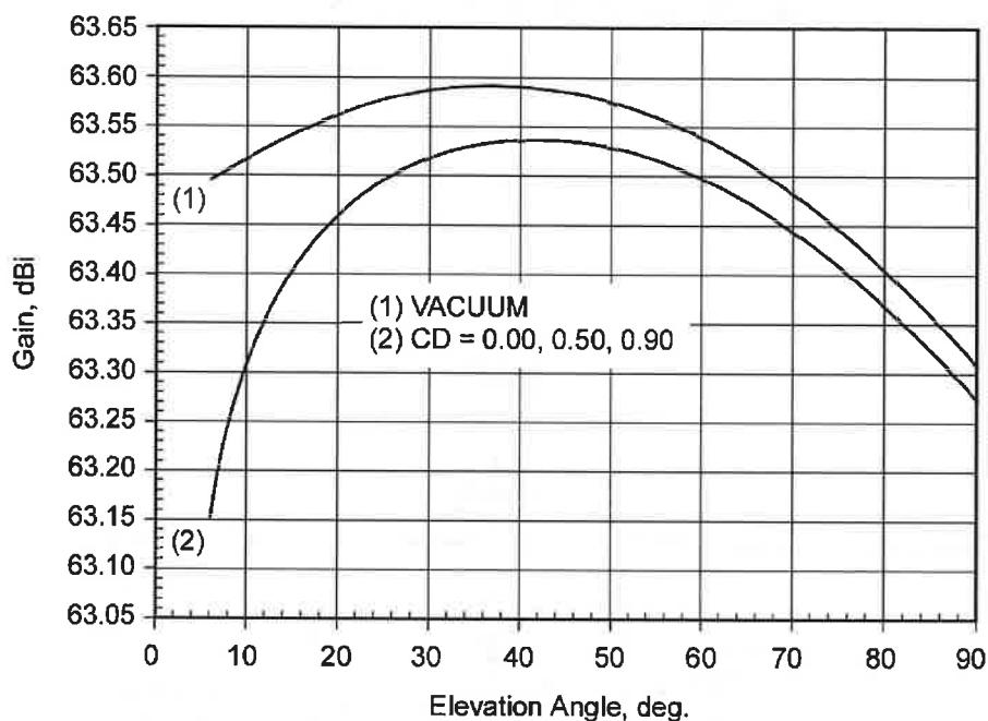
Figure 3. S-Band Receive Gain, All Stations, at Feedhorn Aperture
