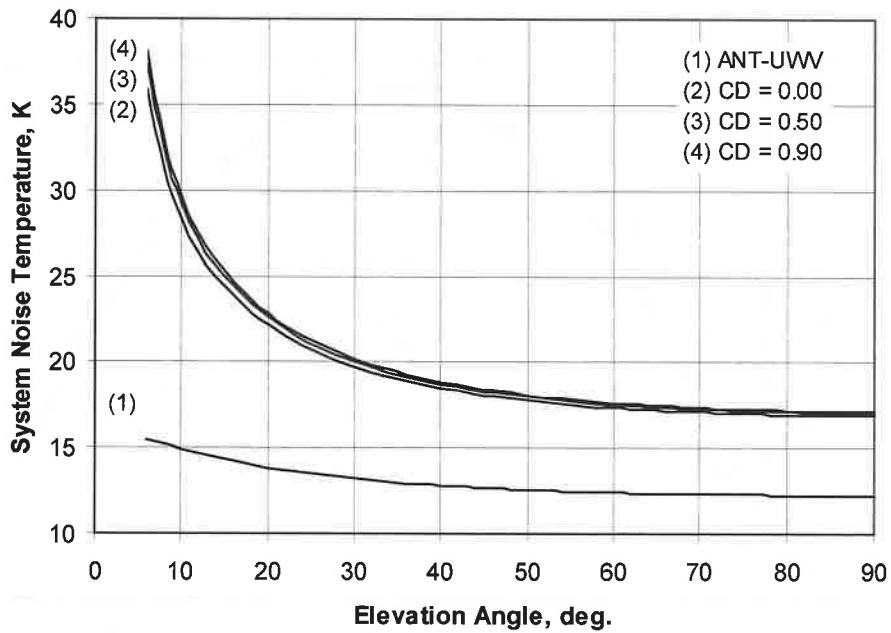
Figure 8. S-Band System Noise Temperature, DSS 14 Antenna, LNA-1,
