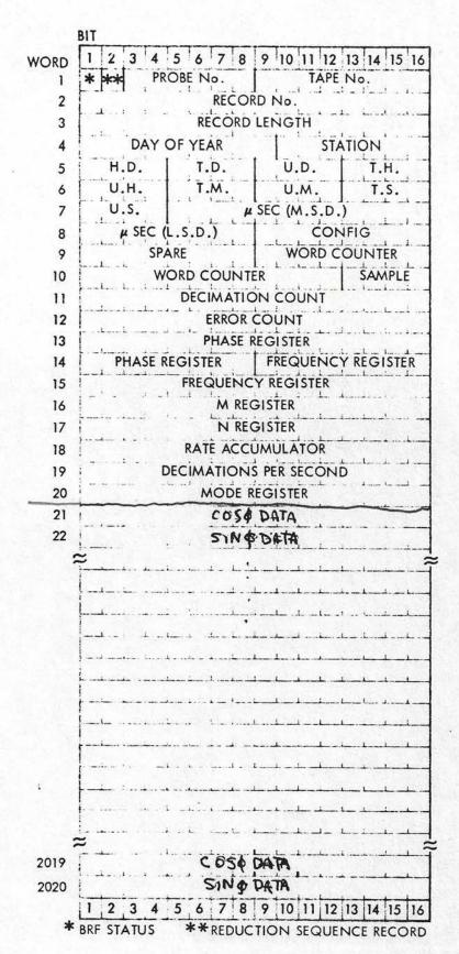
Figure RSC-11-1-1. Wideband Radio Science IDR Block Format
