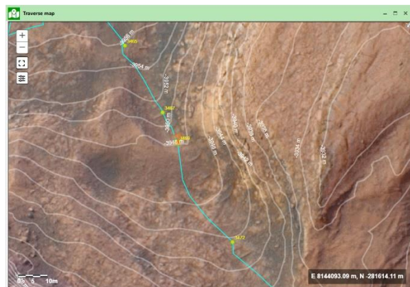
Figure 1. MSL Curiosity AN map showing elevation contours (white), rover waypoints, and drive traverse overlaying a HiRISE basemap.
